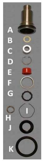
REBUILDING POT BEARING HOUSINGS: The used assembly is disassembled, cleaned and inspected. Epic always replaces the felt sealing washer (B), upper needle bearing (C), nylon spacer bushing (E), lower outer race (F), bearing cage (G), and wire retaining ring (I). Any static parts that show wear or faults are also replaced. The rebuilt assembly is lubricated with Kluber synthetic grease.
